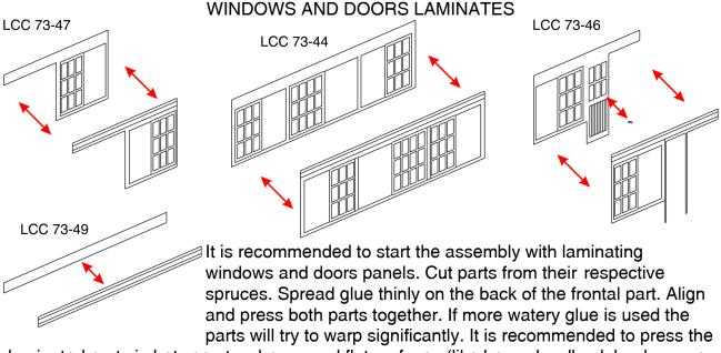
laminated parts in between two heavy and flat surfaces (like heavy hardback books, care should be taken not to allow the laminated parts stick to the books by removing the squezeout [excess glue] and or lining the press with non stick material). When glue has dried the parts will stay flat. Ensure the parts are lined up correctly!
